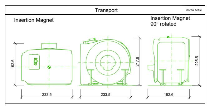
Min. transport opening in the wall: W = 200 cm / H = 240 cmMin. transport opening in the ceiling: L = 200 cm / W = 245 cm
